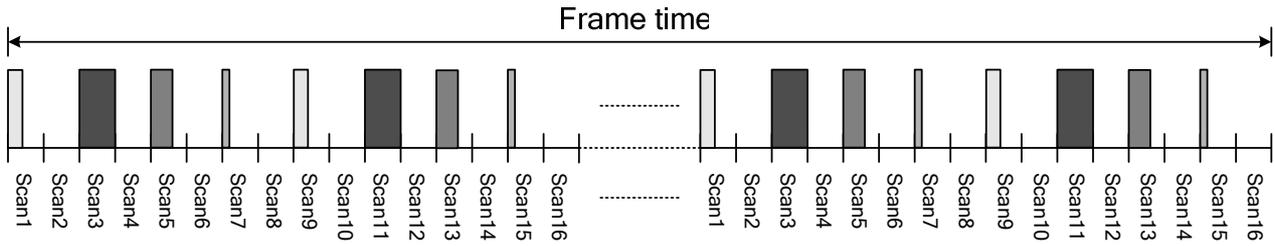
The advanced Multiplex-PDM approach divides the frame time into the designated segments and interlaces Scan images to enhance the refresh rate. By this technique, the frame refresh rate could be improved efficiently by 64 times or 256 times without increasing the frequency of grayscale clock in order to prevent from EMI interference.
