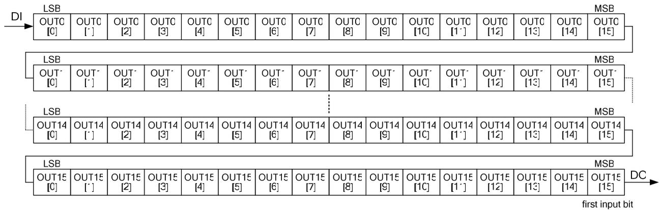
16x16-bits M-PDM data are transmitted into a device for each scan according to the format illustrated above. The first input bit is the most significant bit of OUT15.
