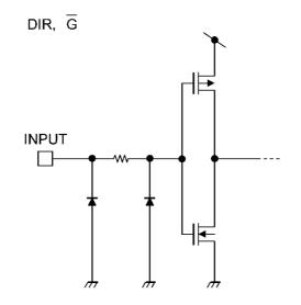
13. Bus Terminal Equivalent Circuit
